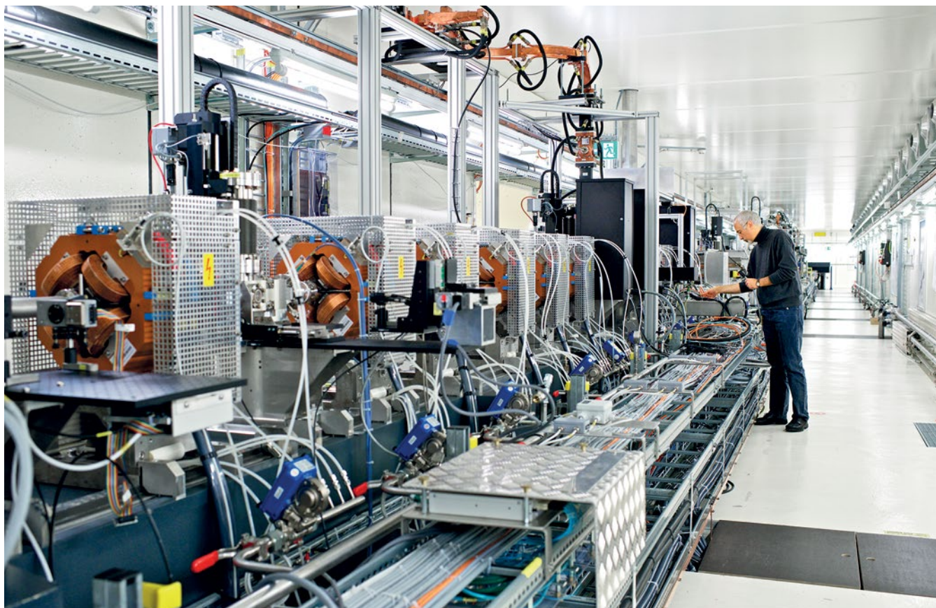
The billion dollar market for accelerator technology is growing year by year. The photo shows the first part of the SwissFEL accelerator with electron source. The 250-MeV injector was set up for test purposes.
