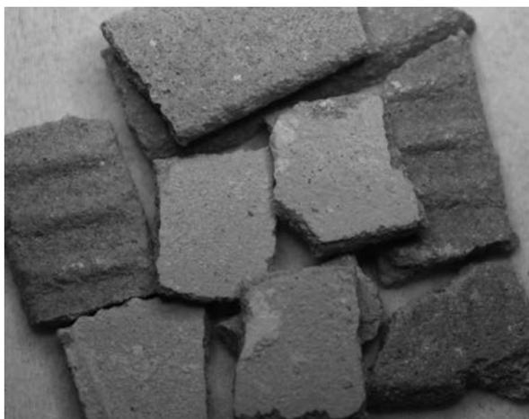
Abb. 7: Asbest in Plattenkleber
